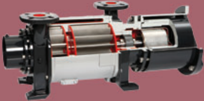
SIHI® LPH-X with magnetic coupling
